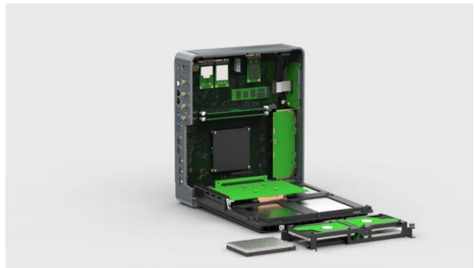
Figure 9 – Install disks and assemble in reverse order
