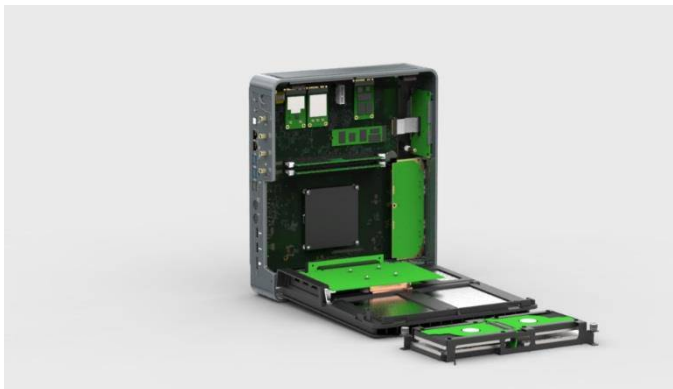
Figure 8 – Pull out the disk cartridge
