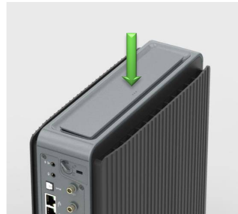
Figure 14 – Press the top-bar
