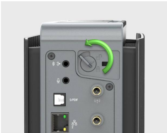
Figure 13 – Move locking knob to open position
